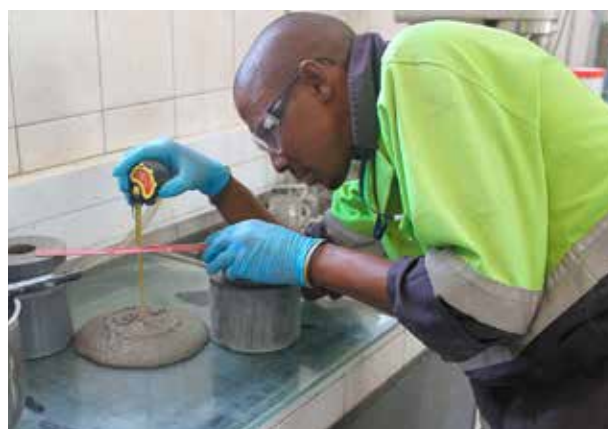
Tumiso Makhubedo doing micro concrete testing at the Centre of Excellence. Micro concrete, unlike a normal concrete mix design, is devoid of all larger particles. It is to simulate concrete workability retention as in ready-mixed concrete applications.
