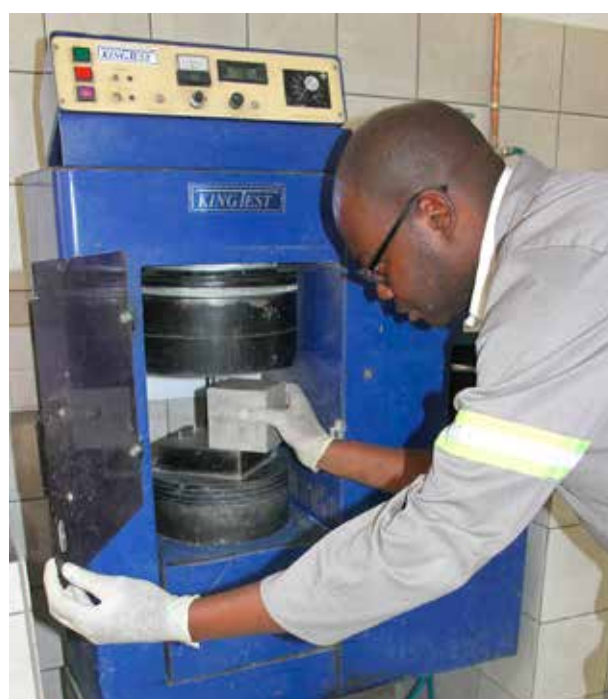
The Centre of Excellence's Owethu Mbeje testing the compressive strength of concrete via the tried and trusted cube crushing method.
