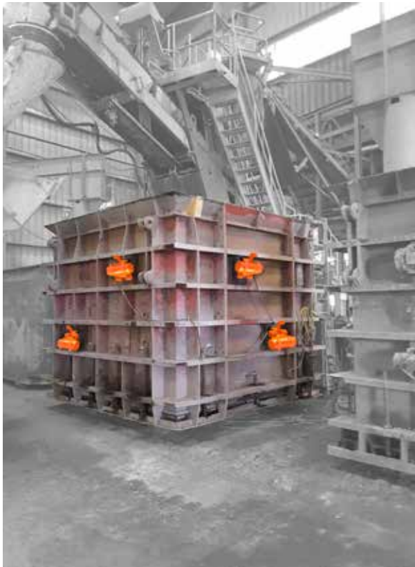
The powerful high-speed vibrator improves material consolidation for exceptional strength and finish.
