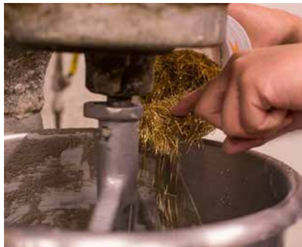
Bronze-coated steel fibres being added to a batch of ultra-high-performance concrete. (Photo: Brittany Greeson, Special to the Free Press)
