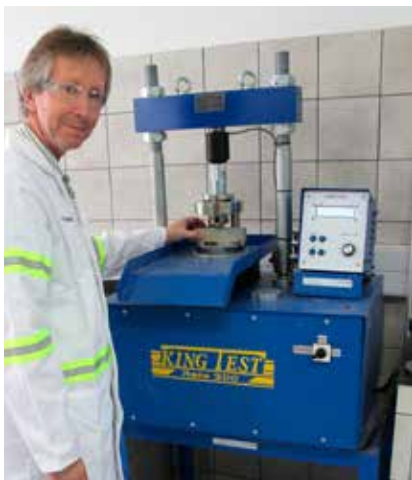
Prism concrete crushing determines the flexural and compressive strengths of cement paste and thin skin liners (TSL). Here Warren Delaney is checking just how much pressure the prism sample can take.
