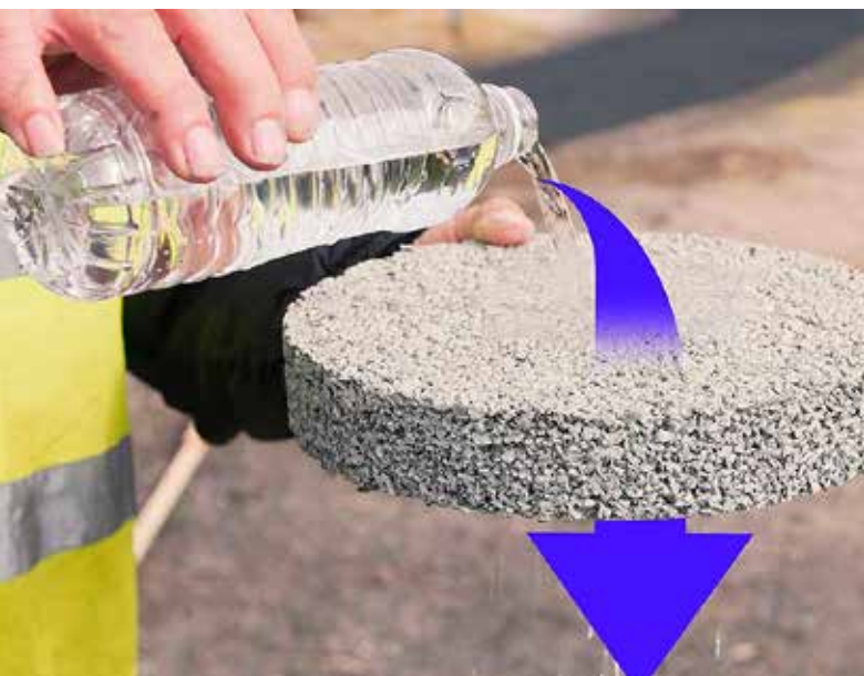
Yellowstone National Park is using porous concrete in all walkways.
