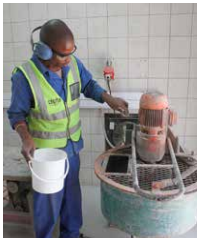
Ithumeleng Mashigo doing concrete mixing to assist clients in formulating the correct concrete mix design for a specific project.
