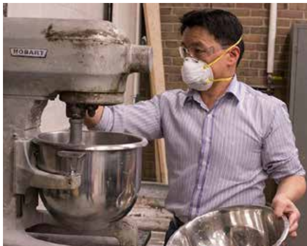
Yu-Shio Tai, a visiting professor from Taiwan and resident expert on concrete materials, adds bronze coated steel fibres to the batch of ultra-high-performance concrete. (Photo: Brittany Greeson, Special to the Free Press)
