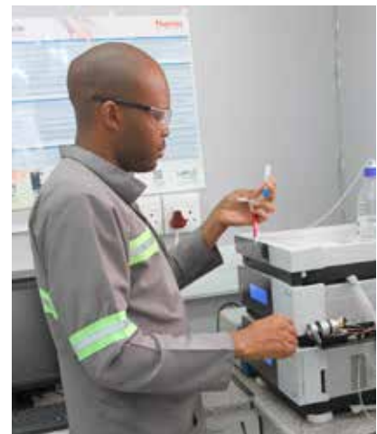
High-performance liquid chromatography (HPLC) testing can separate, identify, and quantify each component in a mixture. Donald Khoza is doing the necessary identification.
