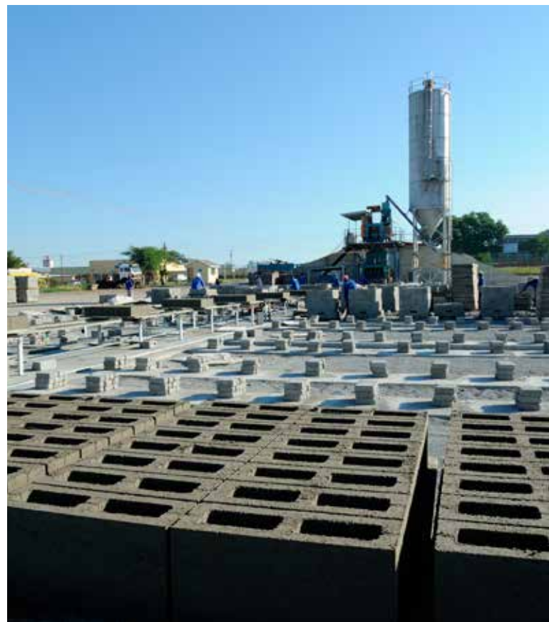
Afrimat's precast factories manufacture concrete bricks, building blocks, brick paving, walling and moulded concrete products.
