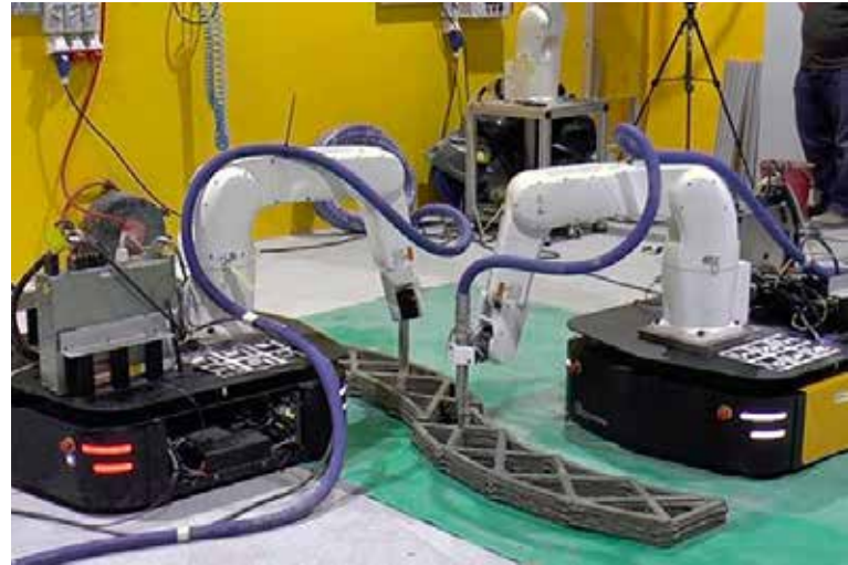
Collaborating robots can tackle different parts of a job simultaneously. Photograph Nanyang Technical University
