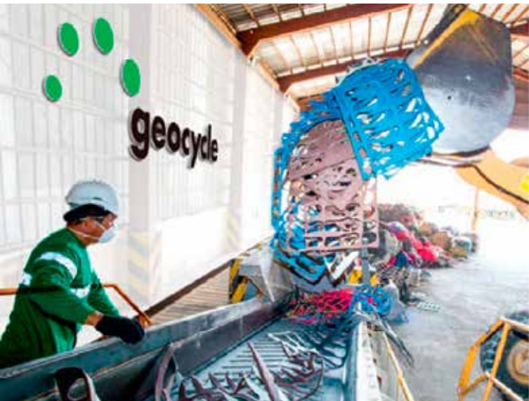
Careful sorting, blending and pre-processing is an essential part of the co-processing of waste.
