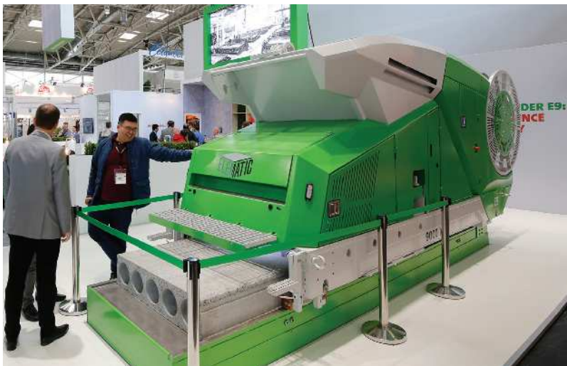
Elematic's Extruder E9 for hollow-core slab production on show at Bauma 2019.
