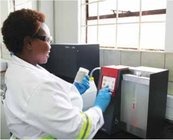
Testing with the electronic air permeability instrument, designed to determine the a-specific surface area of cement.
