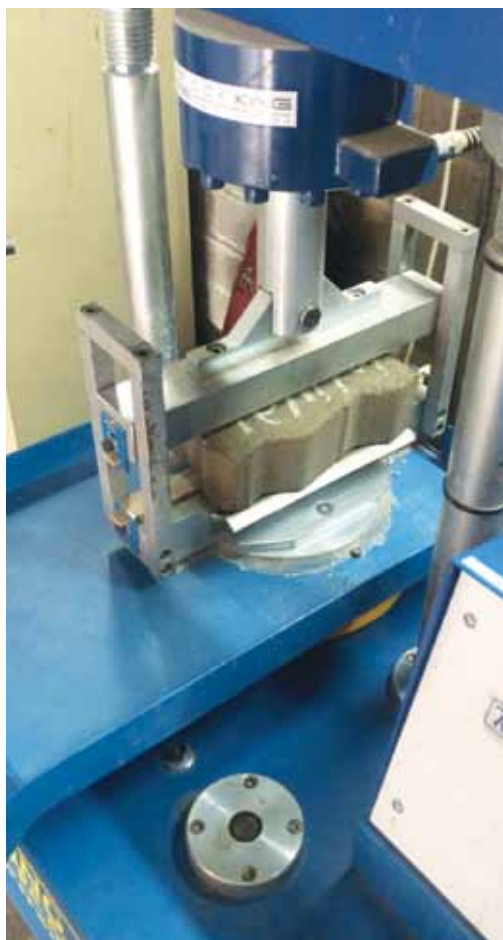
The tensile splitting test.
