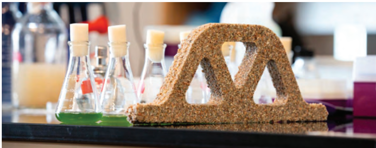
This photograph shows green photosynthetic Cyanobacteria growing and mineralizing in the sand-hydrogel framework. The living material has similar strength to cement-base mortar.
