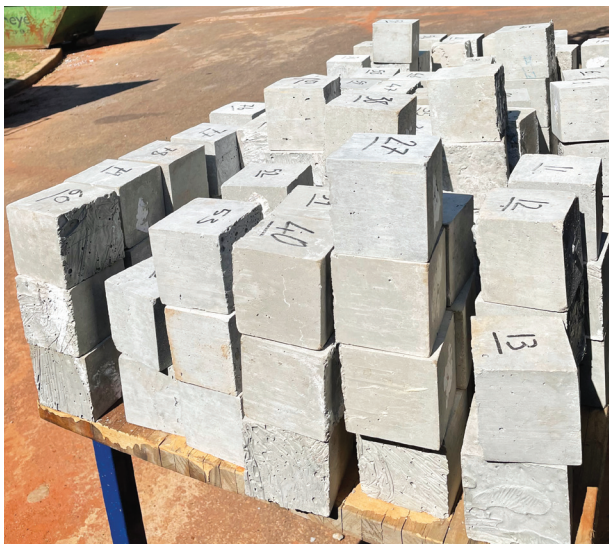
Green concrete specimens prepared by the research partners at the University of Johannesburg
