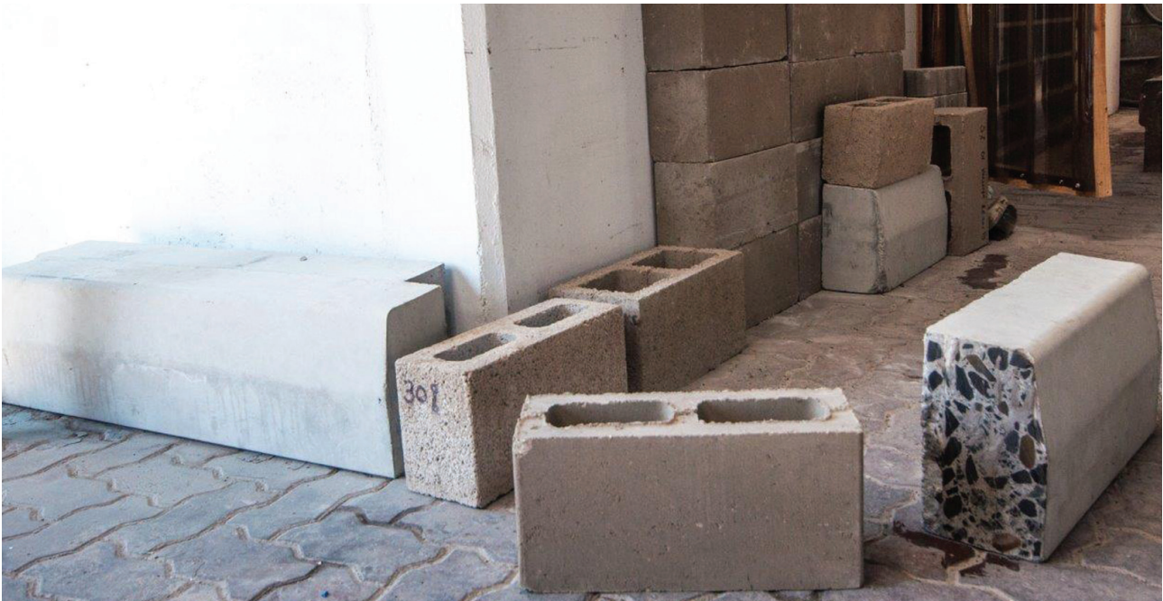
Experimental concrete blocks and kerbs made with varying quantities of RESIN8
