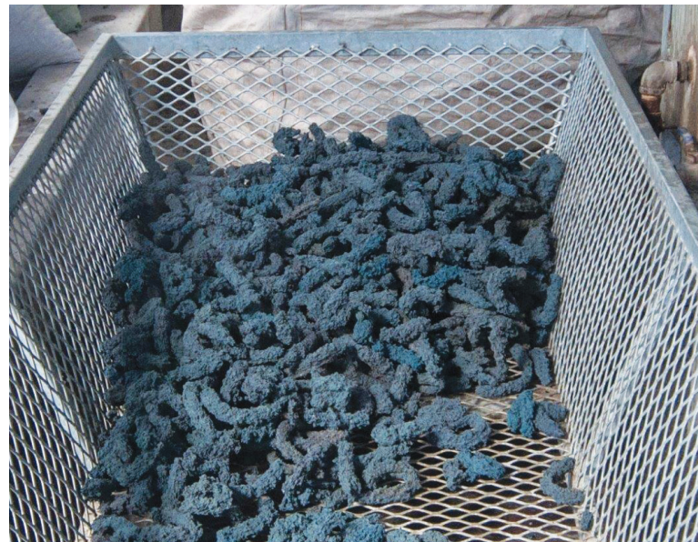
Extruded plastic 'sausages' prior to granulation
