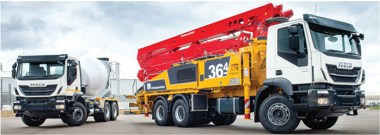
The Putzmeister P6 Truck Mixer and the 36 meter reach Concrete Boom Pump
