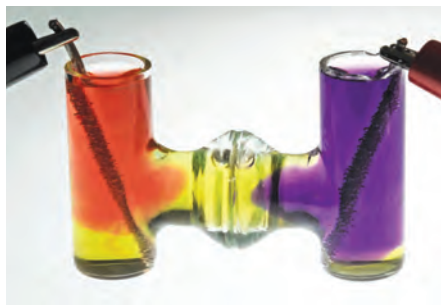
An experiment illustrates the electrolysis process using dye: pink represents the acid created at one electrode and purple the base at the other end. Credit Felice Frankel.
