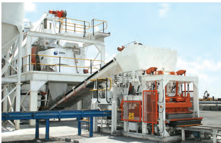
A typical Eirich Birkenmayer brick and block plant layout with an Eirich RV19 mixer.
