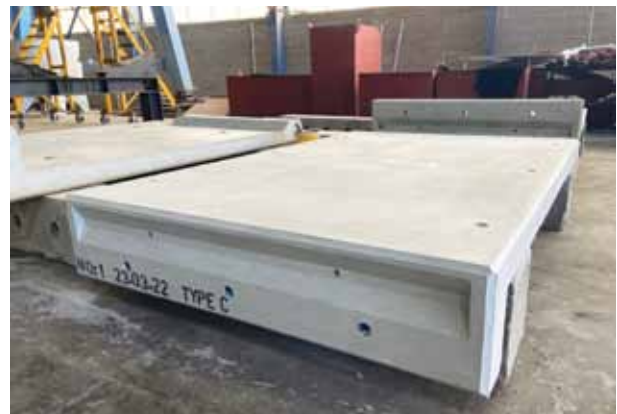
A freshly cast panel showing the V-shaped connection groove at the bottom of the panel.
