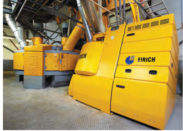
Fig. 1: Eirich mixer for facing concrete at a concrete product manufacturer in Norway
