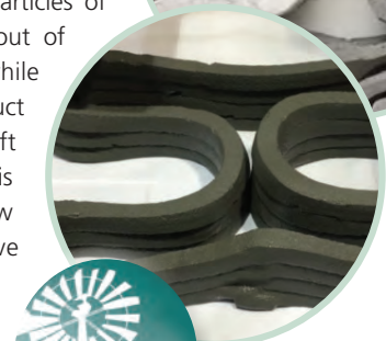
3D printing concrete made from fly ash and steel slag
