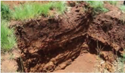
Test pit showing clay soil
