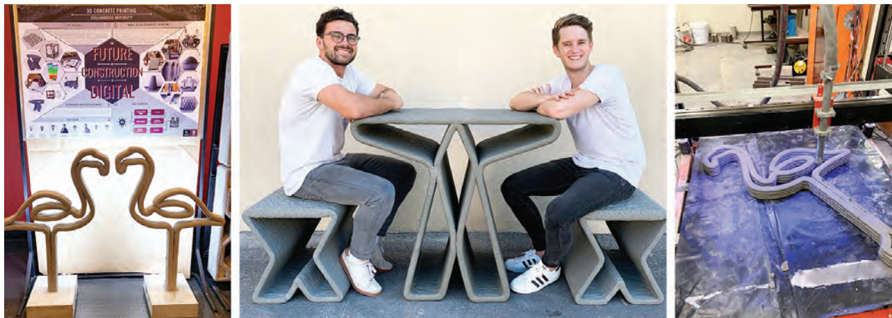
Main photograph: Marchant van den Heever (left) and Frederick Bester with the bench and table X-Furniture prototypes they manufactured by means of 3D printing of concrete. Far right shows the 3D printing process of a concrete flamingo. Far left are the elegant flamingos that attracted many visitors to the students' exhibit at the SA Innovation Summit.
